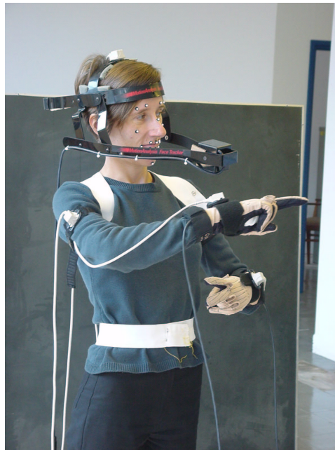
Fig. 3. Data capture: face tracking camera with facial reflectors, Cybergloves for tracking the digits and Polhemus sensors taped onto the back of each hand, upper arm, body and head to track the body.
